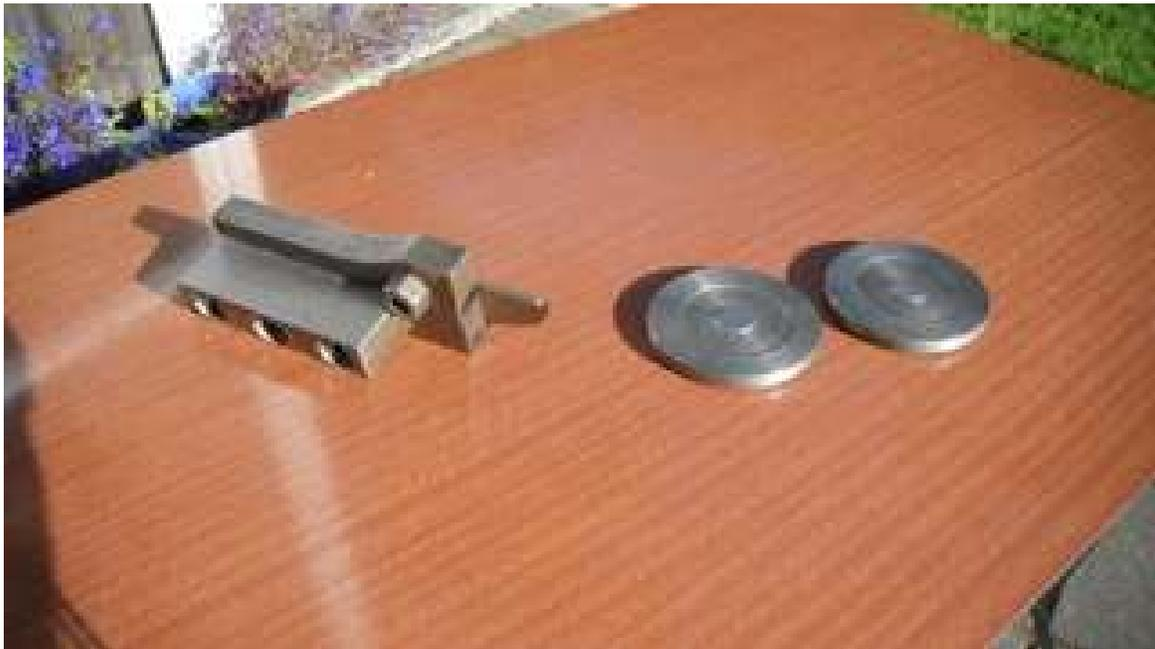
Nigel had a parting tool which had been adapted to fit the tool post on his lathe. This was made from an old holder from a larger lathe. Current work has been making the front cylinder covers for Simplex.
