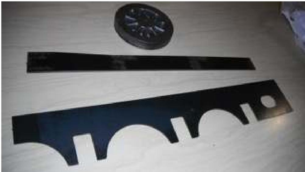
Jim Acott had brought along the laser-cut frame for the Aspinall tender and one of the wheels for the loco, all of which will need to be remade because of the pattern having insufficient allowance for machining. He has found that laser-piercing the rivet holes in the frames is very expensive and is encouraged to try marking out & drilling holes instead. The axle horns are being made at present.
