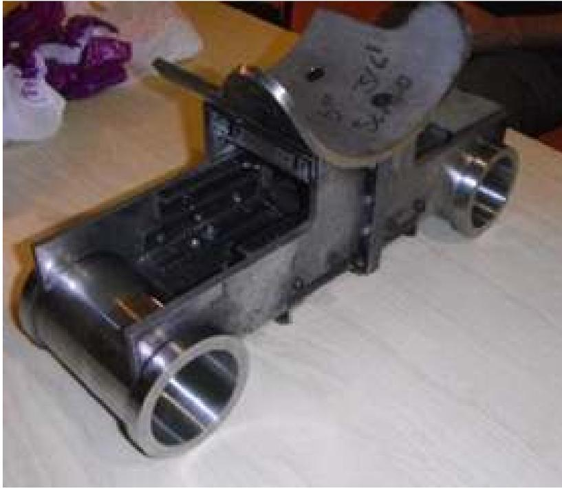
Lawrence Brehaut had the pieces made for fabricating the cylinder assembly for his 7 1/4" gauge 'Q' loco, to show progress. These will be bolted together and final machining of steam chest blocks and porting carried out. He will be fitting bronze or cast iron liners to the cylinders.
