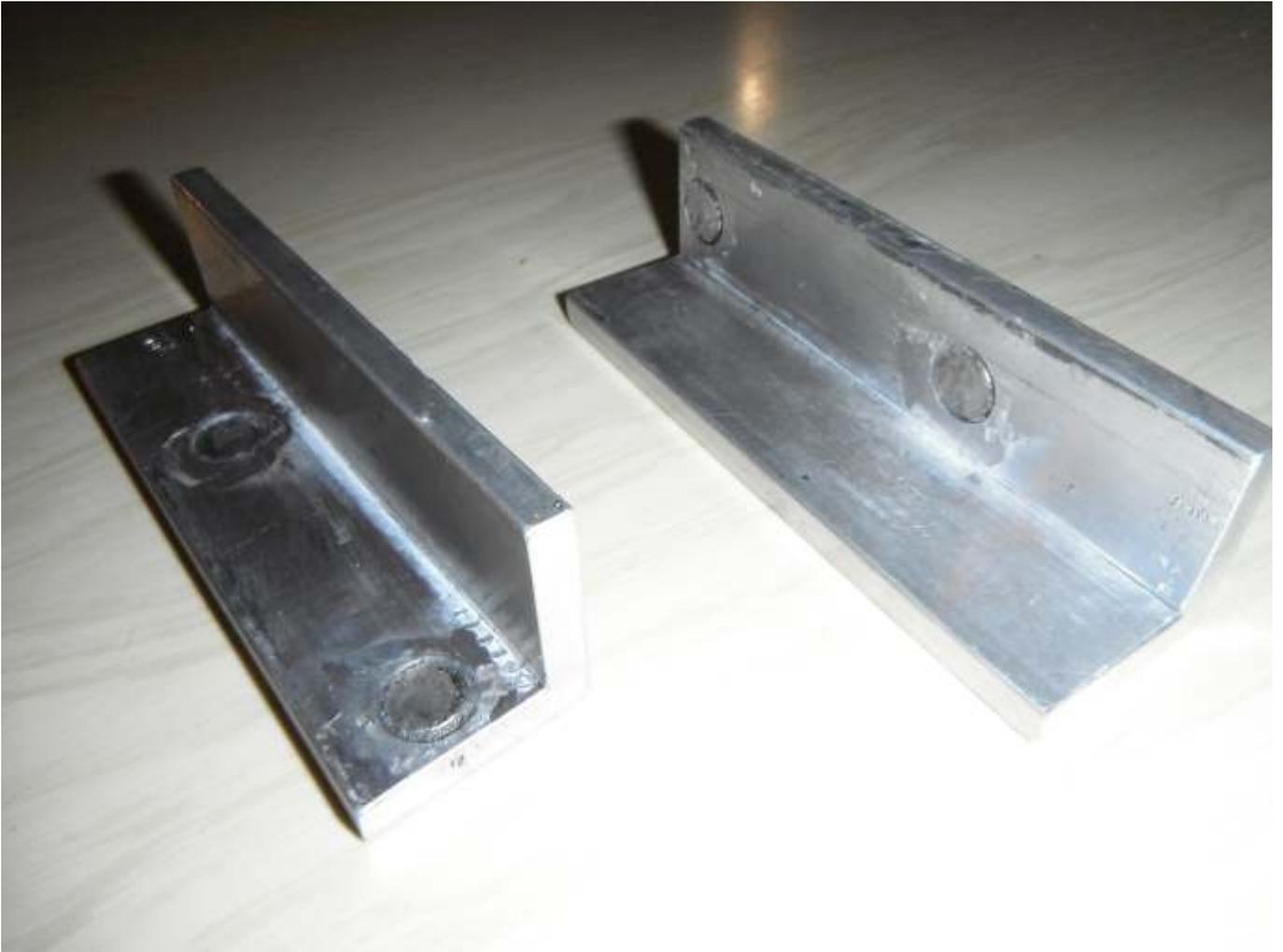
Ron Perkinson had fabricated soft jaws for his machine vice from angle alloy with small powerful magnets inset in milled cavities. A good idea and very useful.
