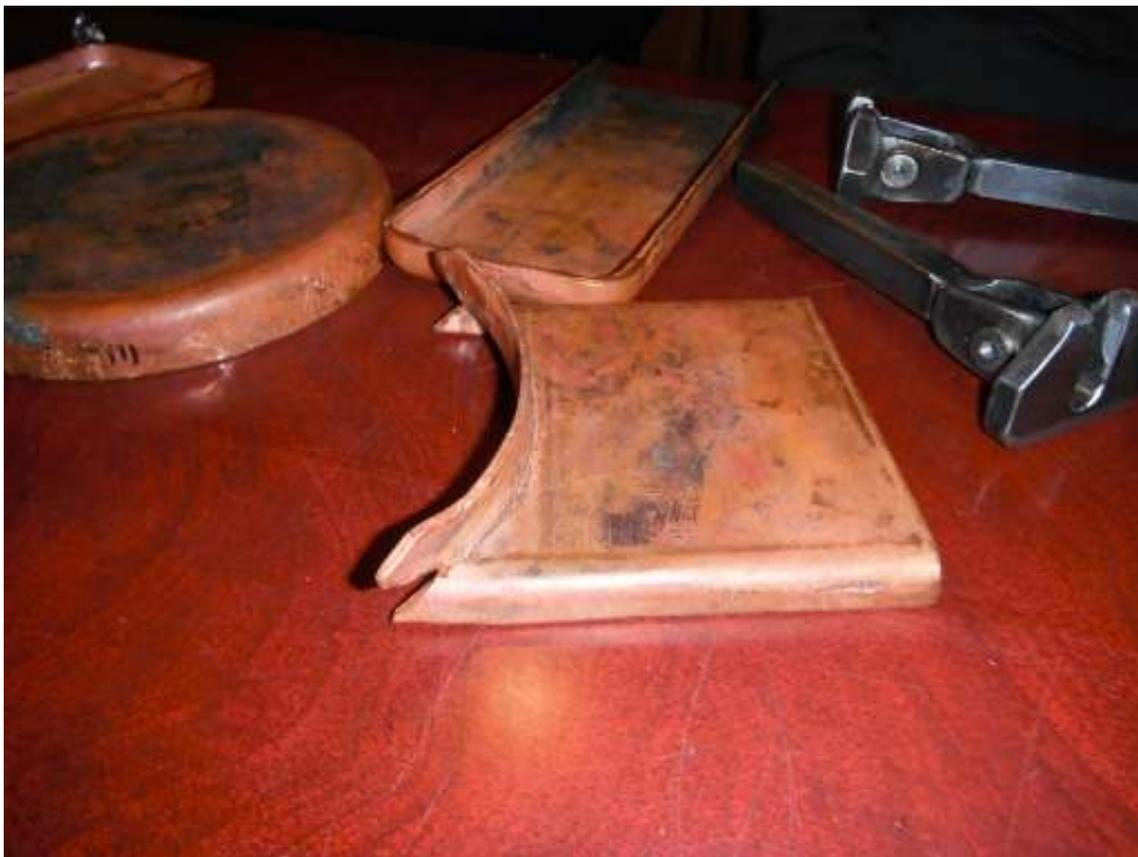
Ron Perkinson showed some of the boiler plates he had made for his Phantom boiler. Very nicely formed. He had two draw bars for the loco as well. There was discussion on marking out and drilling the tube holes in the boiler plates. The subject of easi-flo and the cost involved in fabricating the boiler was also commented on - a cause of some consternation. Ron is ready to fire up his new loco and see if heating would help un-seize the regulator valve.
