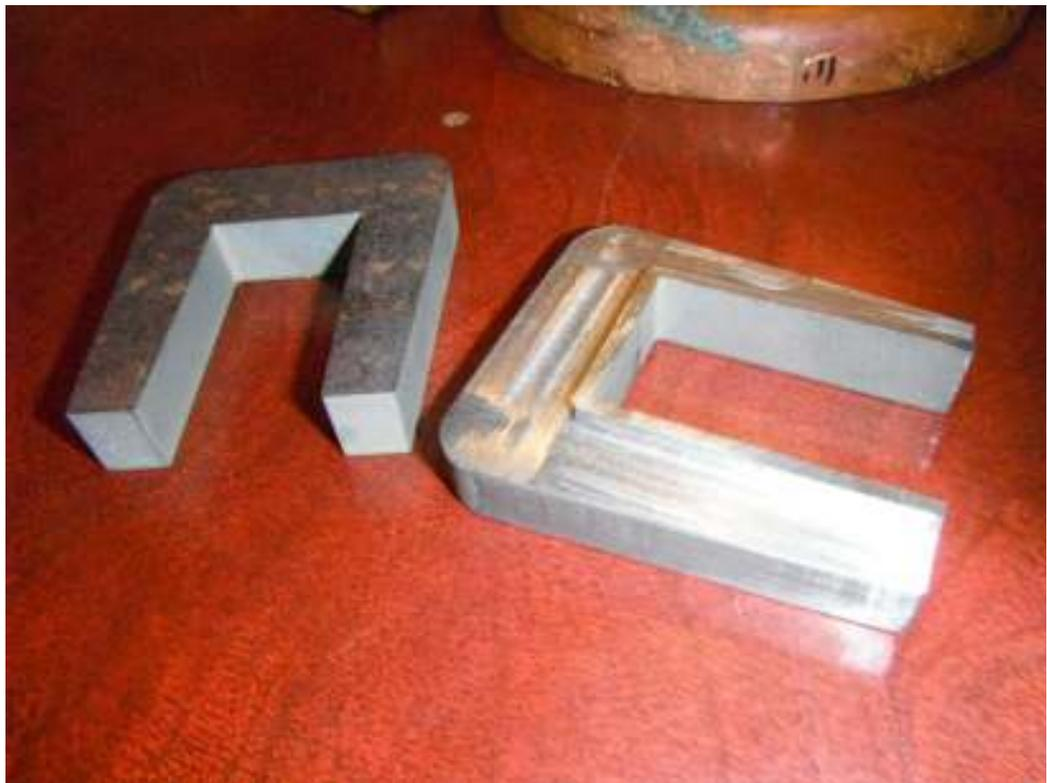
Mark Taylor showed the horn blocks made for his ride trolley which had been water cut. The back faces of the horn blocks were milled to provide a lip for mounting in
