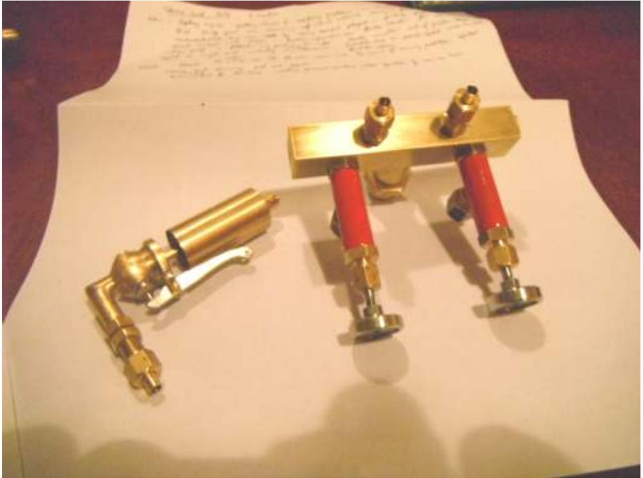
Nigel showed the whistle and steam turret for his Sweet Pea. The regulator valve body that came with the loco needs reworking as the valve spindle seat had been drilled into and didn't provide a sealing face. Suggestions offered to aid in recovering existing valve body.
