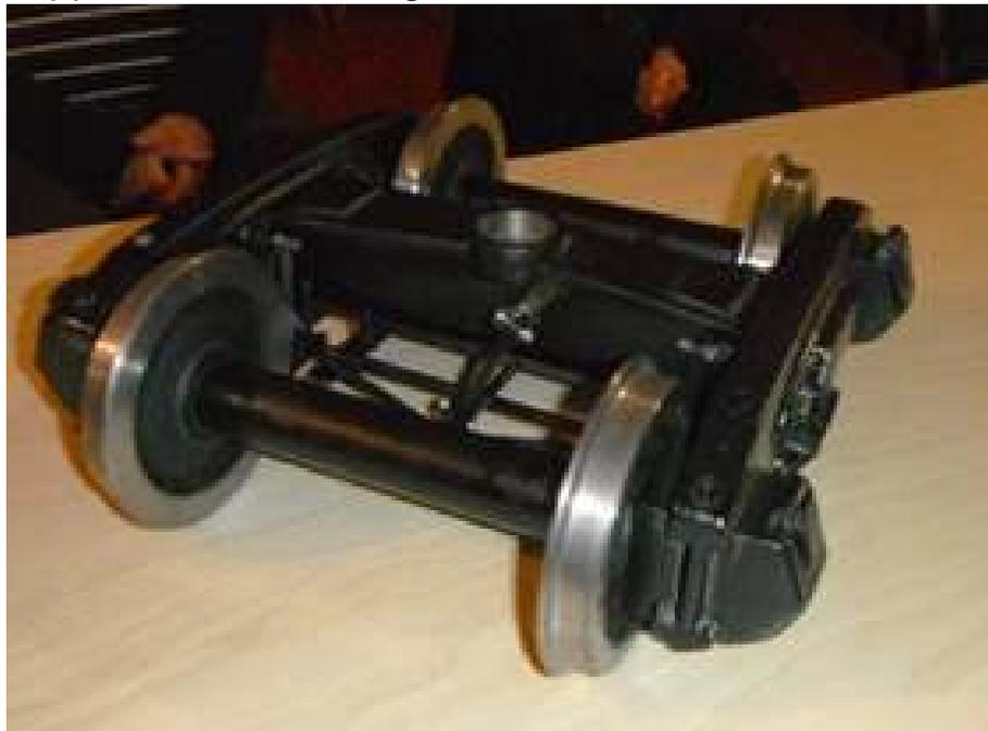
Win Holdaway had a truck assy for the driving trolley for his A5 Pennsylvania shunter. This will house batteries, compressor, etc. The truck frame had been cast in one piece.
