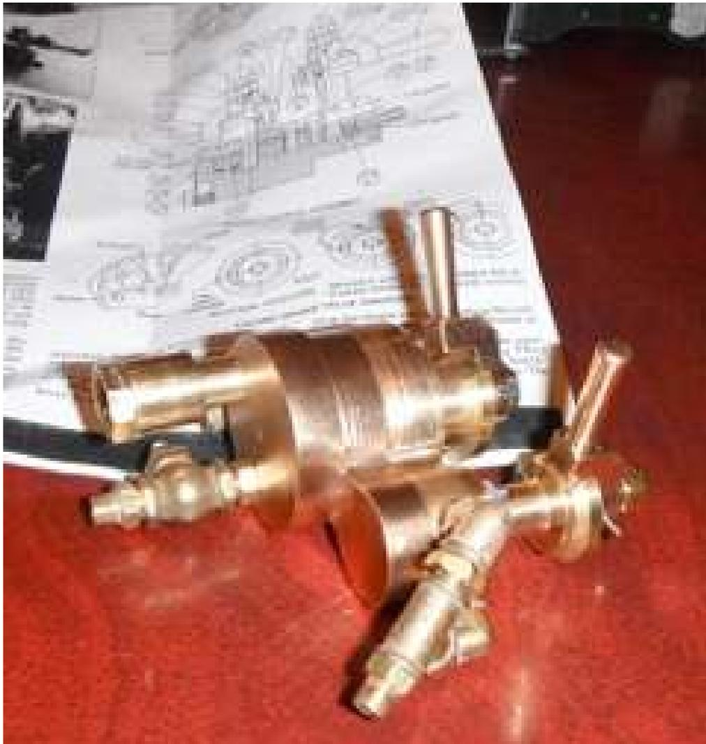
Win Holdaway has been making the brake operating valve for his 7 1/4" g Pennsylvania shunter. It is a Westinghouse type and he wanted to make a fail-safe operating system. The unit is beautifully made and required fabrication of several specialised tools for turning parts.
