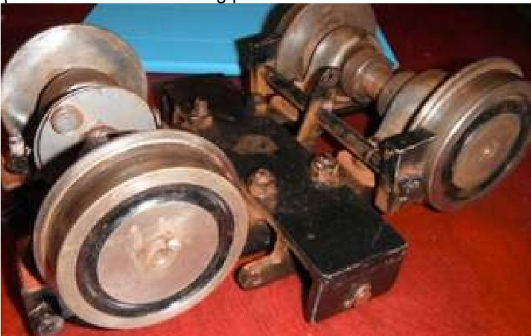
Nigel has been working on improving the brakes on his driving trolley which was purchased with his Sweet Pea loco. There was braking on only two sets of
