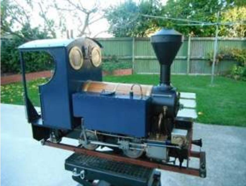
Nigel Wood has been making a spark arrestor for his Sweet Pea after getting cinder burns. Making the base collar for the chimney from a brass billet has been interesting. A plug was cut from the centre of the billet by water jet to save a large pile of expensive swarf in the machining process and the collar just needs to have the radiused section finished off. It remains to be seen how effective the new chimney will
