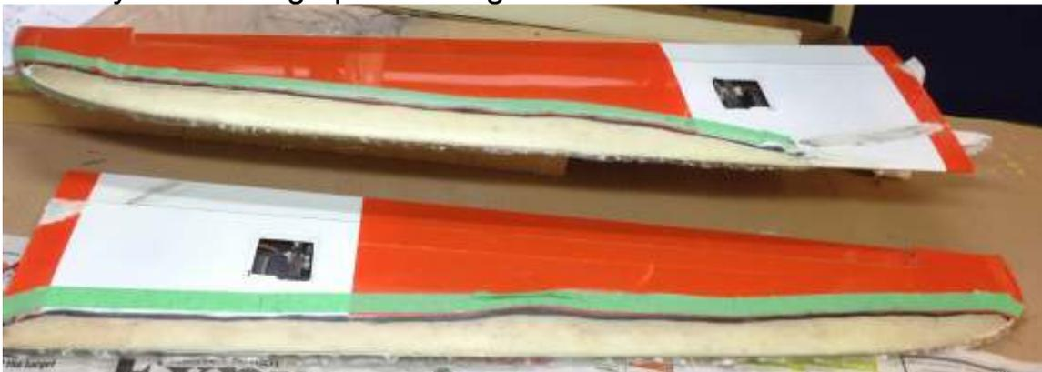
*The Superior tip panels have the leading edges filled with foam, shaped then glassed.*
