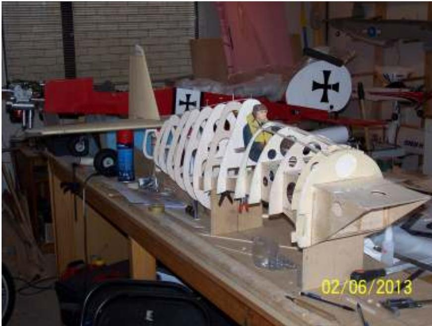
My long term design and build project, the 1/6 scale F6F Hellcat, has progressed a bit further with the forward fuselage internal structure from front bulkhead to the wing seats built, and all the fuselage frames cut. Working on the Tailwheel retract mount. Previously I built and covered the Vertical Fin and Tailplane.
