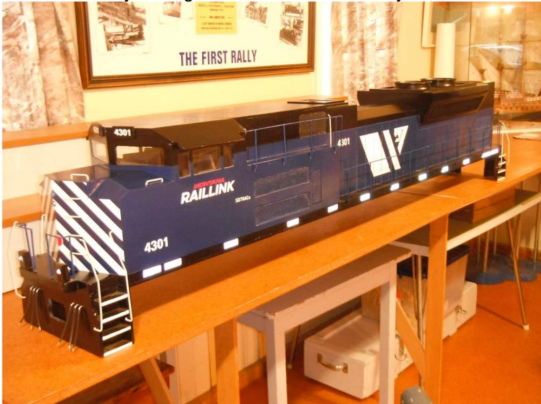
**Allister Green** displayed the bodies he had scratch-built to be fitted to his 5" gauge English Class 66 loco chassis. These bodies are made to scale using MDF
