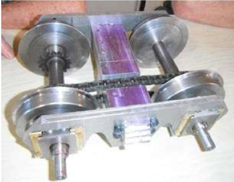
On the table was a bogey assy under construction by Mark Taylor for a 5" electric powered locomotive. This will be chain driven by motors mounted on each bogey. Needle roller bearings in the axle boxes.
