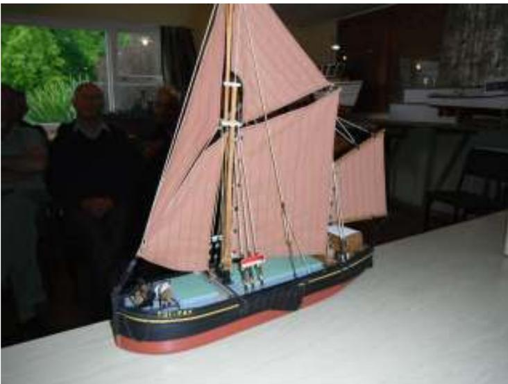
Boats: Graham Vercoe had completed building a freescale model of a Thames sailing barge from a photograph. Of balsa construction with single channel r/c and sails reasonably well with a plug-in keel. Looks very realistic.
