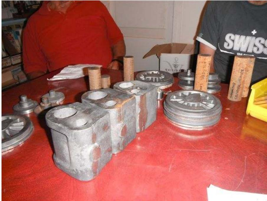
Mark unpacked a heavy box containing wheel and cylinder castings for his Speedy and cylinder castings for Ron's Springbok. Very nice castings from the UK. Ron Perkinson had problems with corrosion in the side water tanks for his PV Baker (made from zincalume or similar) and which needed replacing. He showed the parts he is preparing for fabricating new side tanks.
