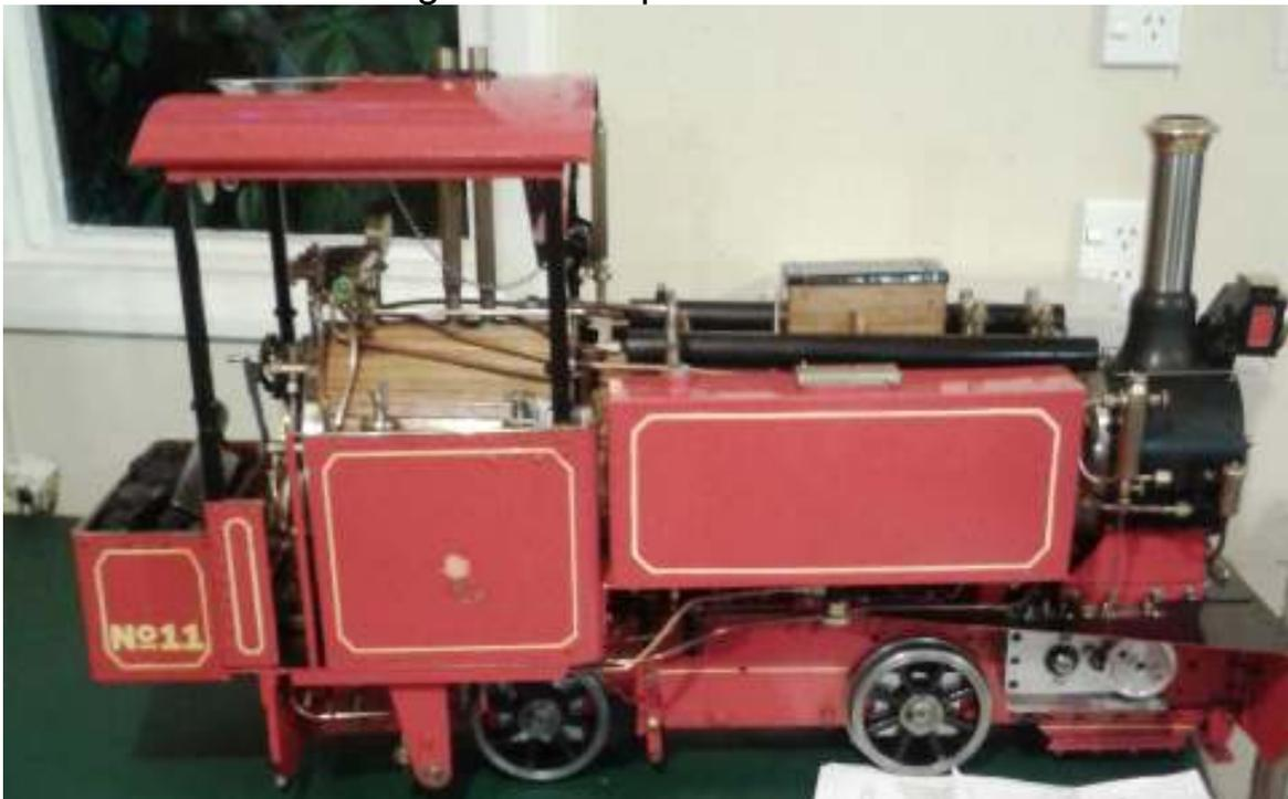
Ken McIntyre had his completed Tesla turbine powered locomotive and described the problems he had encountered during course of construction. It did not come up to some expectations in that it needed a lot more steam than the boiler could generate but works well otherwise.
