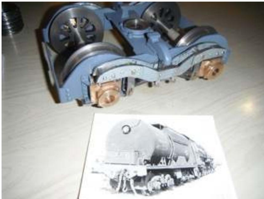
John Bolton had one of the completed bogies for his 3 1/2" gauge NZR Ab loco tender and was working on the second bogies plus the brake system.
