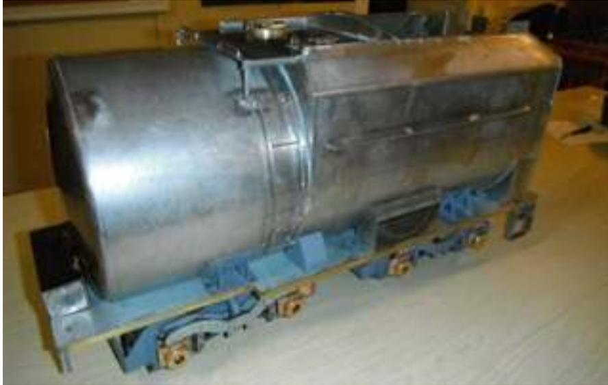
John Bolton showed the assembled tender for his NZR Ab loco which he had bolted together for the first time, finding a few challenges along the way because some components were obstructing access for fastening other parts. It looks good but he would like to finish the tender before starting on the locomotive.
