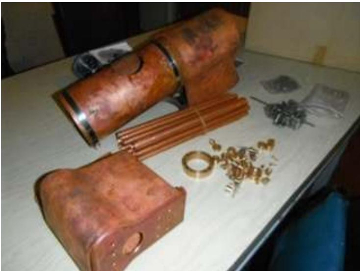
Jim Acott has been busy producing bits for the tender suspension on his Aspinall locomotive and had brought these plus several formed plate and other components for the boiler.
