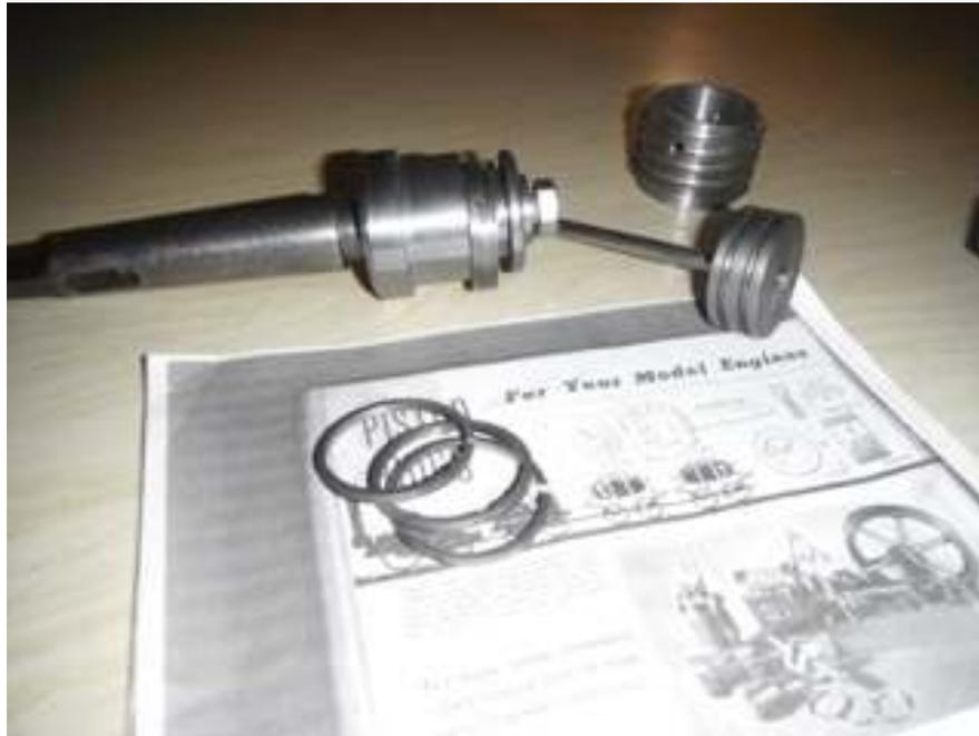
Nigel had been making piston rings for Simplex which involved fabricating a holding fixture. An interesting exercise.
