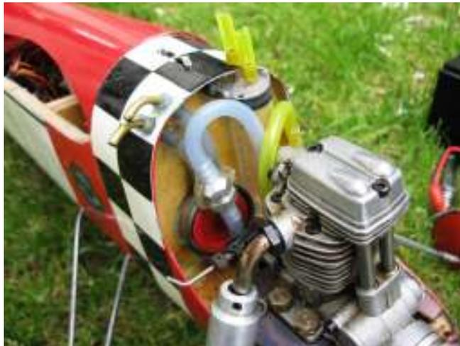
*Lancer engine bay setup for both A and Open Texaco*
