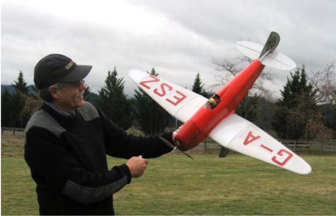
*Chilton from 1949 Aeromodeller plan scaled to 42 inch span and powered by the ubiquitous Cox BabBee tuned and propped for long engine runs.*
