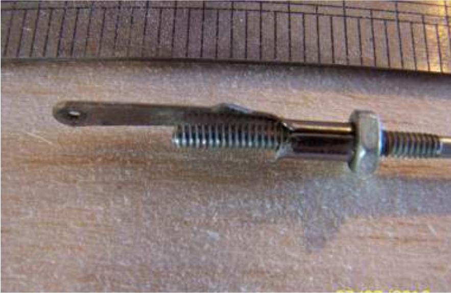
Late on Sunday I had a steel Quick-link break on the left flap control rod, which lead to some odd handling problems when I lowered the flaps for landing but after an overshoot and raising the flap it landed safely. It was a Great Planes 4-40 steel quick-link and one side broke off completely. One of the other flyers says he lost a model when one of
