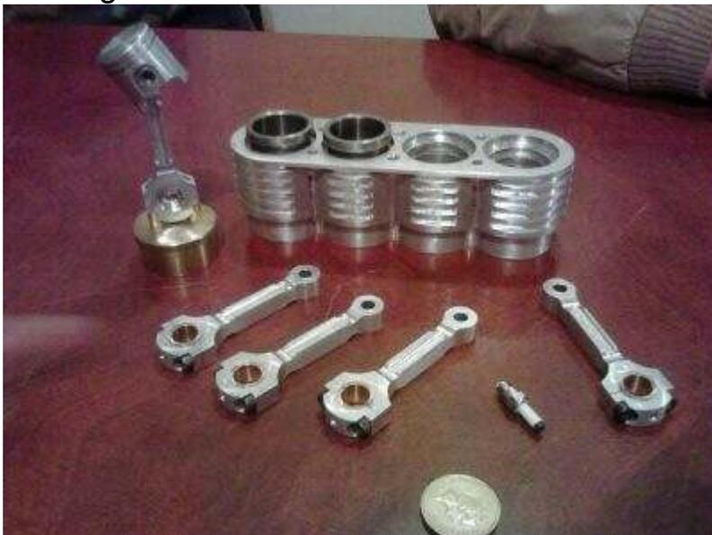
Brent Coburn has been making the con rods for his 4 stroke marine engine – profile was cut out with high pressure water jet cutter and then machined. He has made the pistons and the cylinders, which have been modified for water cooling, are under construction. Cylinder liners are made from cast iron. Cylinder heads and valves being machined. Using commercial
