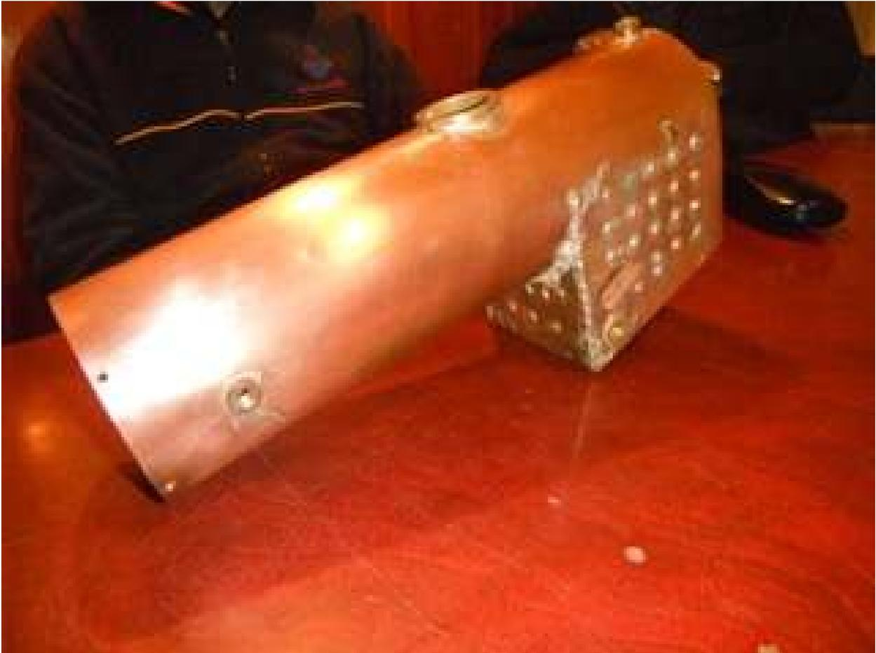
Lawrence Brehaut had the boiler for his 5" gauge Boxhill made some 30 years ago but never tested. It was made to Martin Evans published 1964 drawing before the ABMSC code was adopted. All parts for the loco are made but some checking is needed as adjustment of valves is suspect.
