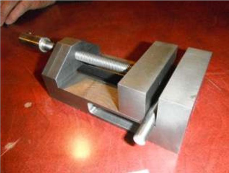
Ron Perkinson has made some more progress with the replacement water tanks for his new loco. He showed a machine vice he had finally finished after 30 years. It is made from castings and was an exercise in metal work but will be very useful.
