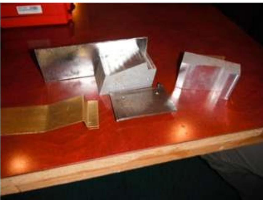
Win Holdaway showed a die he made for pressing a series of steps in sheet brass for his Pennsylvania loco tender. The die was extra work but ensured that each step would be uniform.
