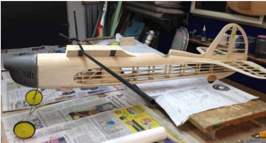
The model is taking shape in my workshop. I'm thinking of a US military trainer scheme like my Scram except with the Dark green fuse used on the Curtis Hawk 6. The Carbon tube will be the wing spar. The outers plug into a centre section.
