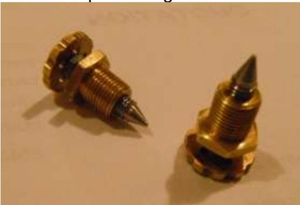
Tom Hood has been helping Murray Hewetson by making sight glass blow down valves for Murray's 5" gauge Britannia. This has been repaired and is nearly ready for steam trials again. Discussion on methods of cutting tapered valve faces on threaded spindles was interesting.
