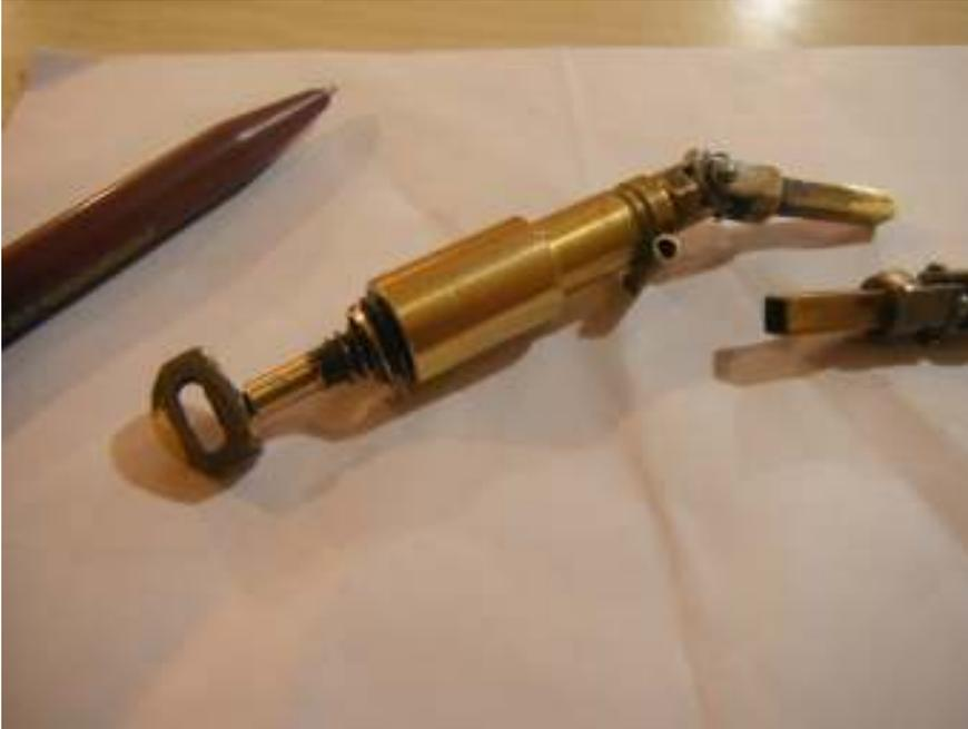
The set-up was erratic and very sensitive to curves in the track - curves one way would close the throttle and vice versa for curves the other way, so he developed a control mechanism with left-hand and right-hand threaded internal parts which would extend and retract to give the required throttle movement with minimal rotation of a control wheel on the back of the
