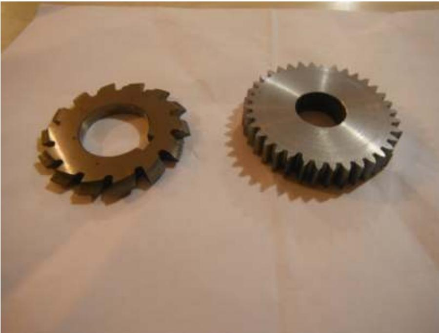
a modular cutter and queried how to determine the depth of cut. This is usually shown on the cutter but was hard to decipher. In discussion which followed various points were noted such as selecting the correct cutter, the outside diameter of the gear is critical and the depth of cut is important.
