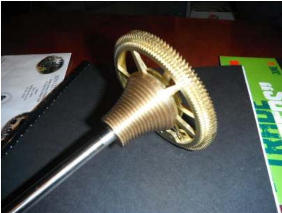
Murray Brown has been busy on his clock project and showed progress on the fusee shaft and gear wheel with spring loaded ratchet which maintains power to the gear train. He cut the gear teeth with a cycloidal cutter and the ratchet teeth with a radial saw blade. He had to fabricate a back gear train to obtain a suitable speed and torque for cutting the large gear wheel. He will be using cord on the fusee rather than chain
