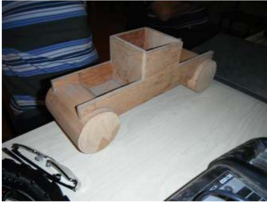
Lawrence Brehaut had brought along a mock-up of the cylinder unit for a 7 1/4" gauge NZR 'Q' loco and asked for advice on whether to fabricate the cylinders unit or to make a mould and cast as one piece. In discussion it was considered that fabricating cylinders and the surrounding structure and TIG welding together would be most practical. The cylinders could be bored and sleeved after welding.
