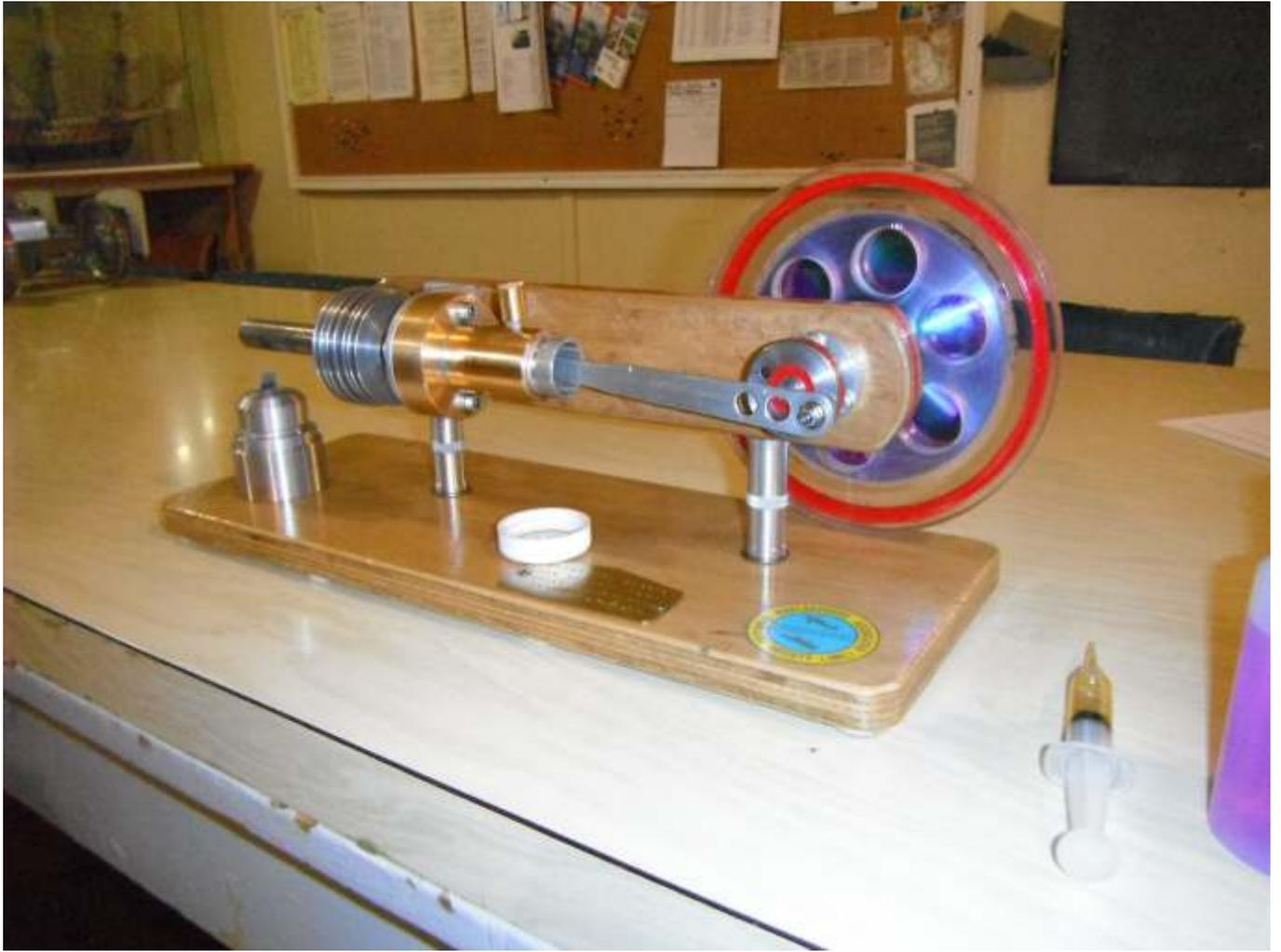
Ken McIntyre has made a horizontal Stirling hot-air engine and it was fascinating watching it operate. He had problems getting it going but determined that clearances between piston and cylinder were too neat. He added a lubricator for the piston using light machine grade oil which improved the situation markedly. There is a 50 deg C temperature difference between the ends of the heat exchanger.
