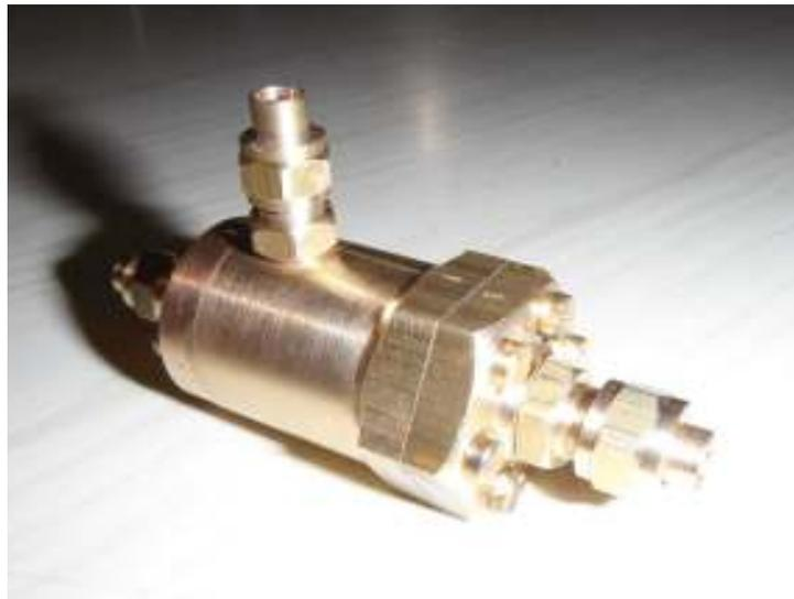
He also showed a triple valve he had made for the brake system. This is a simplified Westinghouse valve and is a form of fail-safe brake operating. There will be a triple valve on every bogey and a pneumatic reservoir.
