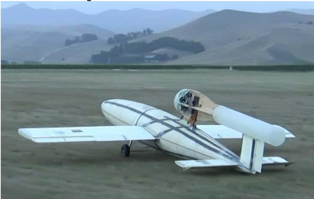
Naked in the early dawn on the runway for the first time. Tricky on the two wheeled gear with no airflow over the tail controls from the 5 high mounted electric fans. (60 Pounds of thrust)
