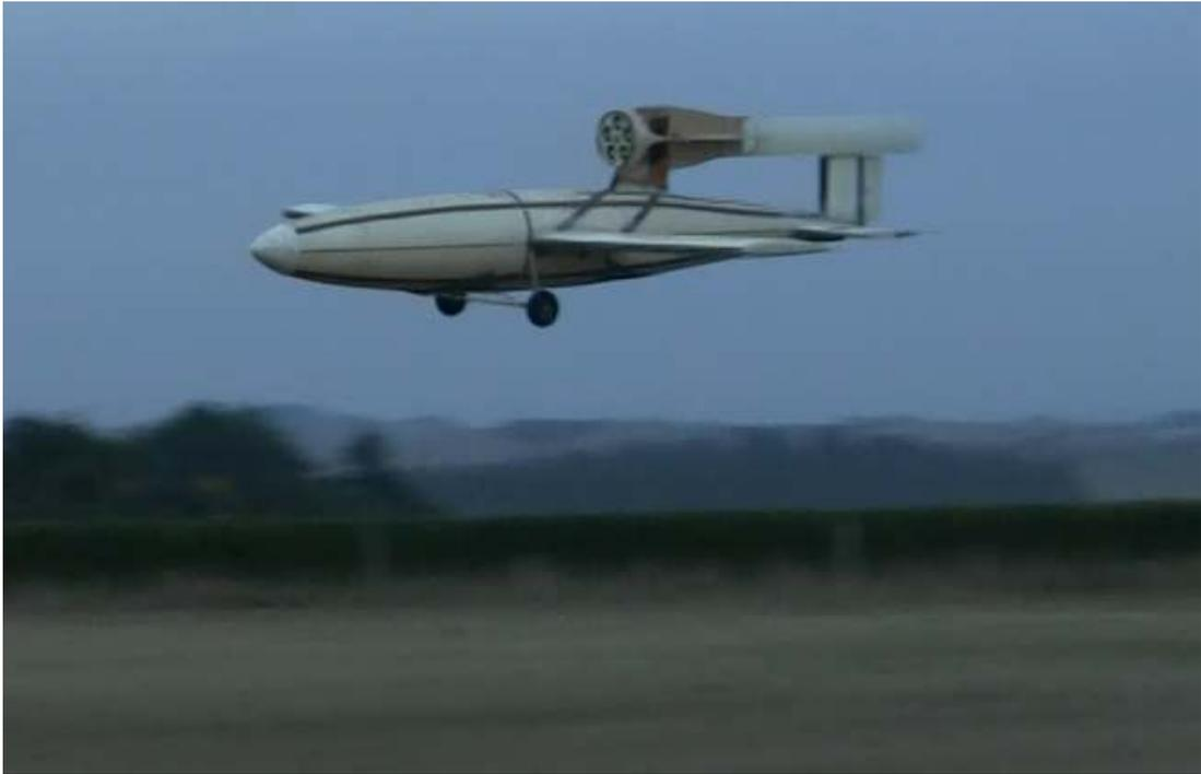
On approach for the first wheeled landing. I found it a bit challenging and bounced to varying degrees on all landings. Forward placed and stiff gear meant it needed to be perfectly 3 pointed to avoid this. Fortunately no such problem for Andrew on the belly landings.
