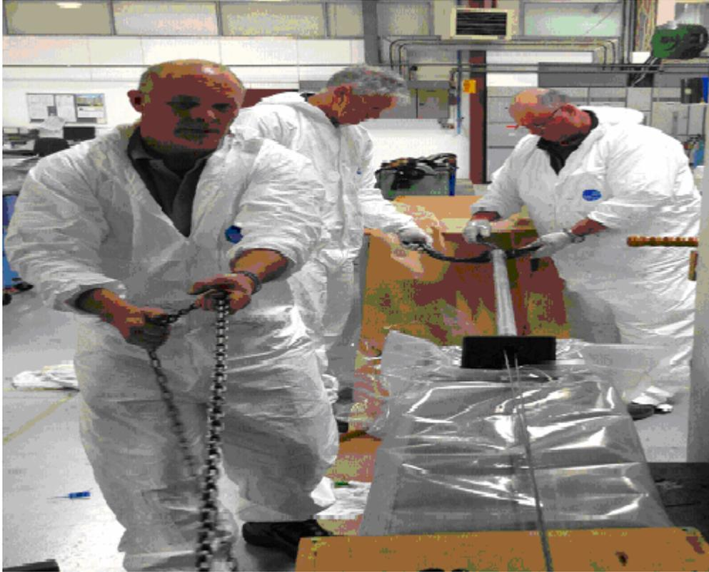
Shane pulling the wetted out carbon units for the 35 mm diameter solid carbon wing joiner. It took a 1.5 ton chain block to pull them through the aluminium forming tube and fire extinguisher to cool!
