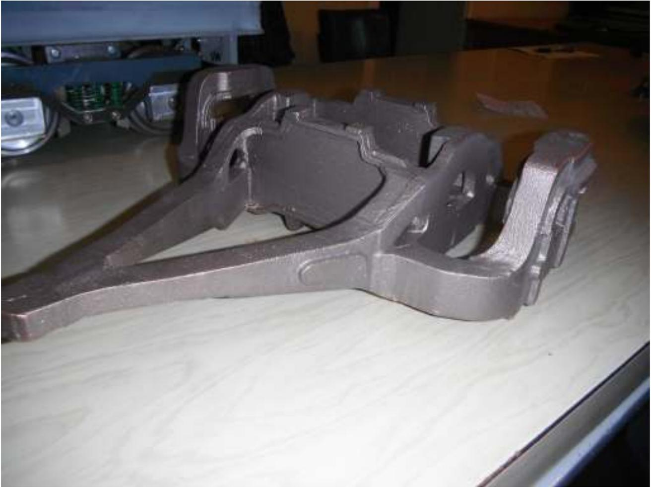
Win Holdaway showed the casting he had recently made of a leading truck for an American locomotive. The pattern was made of high-density polystyrene which was coated with a ceramic compound and treated as for a lost-wax casting. The ceramic coating was applied in multiple layers then heated to remove the polystyrene and calcify the coating before filling with gun-metal while the ceramic was still hot. He made two of the castings for a friend.
