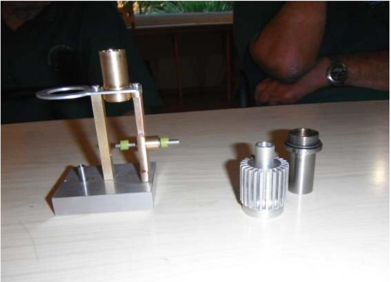
Ken McIntyre showed the small project he is currently working on - a miniature ring bottom hot air engine. This is very light in construction because of weight limitations and runs on meths. He showed the hot and cold ends and displacer. The cylinder with piston to be made. He is using very small needle roller bearings and plans to put the finished motor in a boat as it should have up to 11 watts output at 700 - 800rpm.
