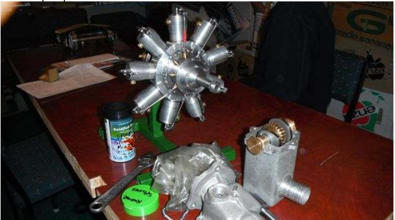
He had been loaned this pump from which to take dimensions. He is making an improved bearing mount for the pump drive to give better bearing wear. The full-
