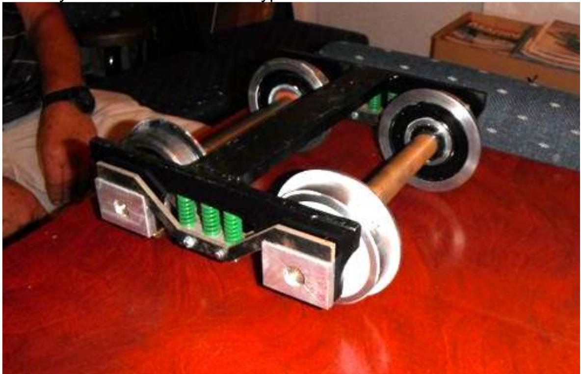
This has to have brake gear fitted and each wheel has independent bearings. He has been experimenting with a Baldwin-type cow catcher and had made a very nice looking bell to mount in due course.
