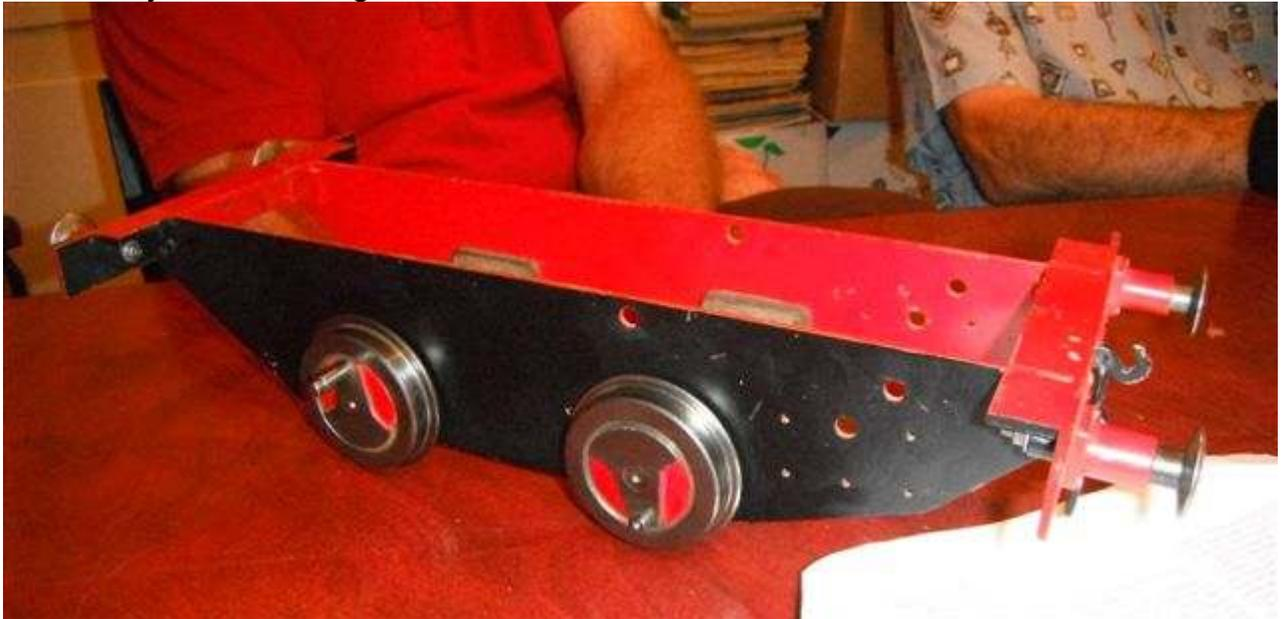
It was good to see John Neal who had brought along the rolling chassis for his 3 1/2" gauge Tich which requires some rework of coupling rods. He has made a start on machining the cylinders.
